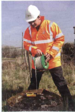
Pinpointing gas migrating beyond the site's boundary, where it can cause the most harm, is of particular importance
