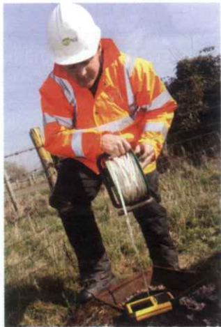
Pinpointing gas migrating beyond the site's boundary, where it can cause the most harm, is of particular importance
